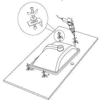
Step 4 Screw the total part on the top and strengthen the part C
